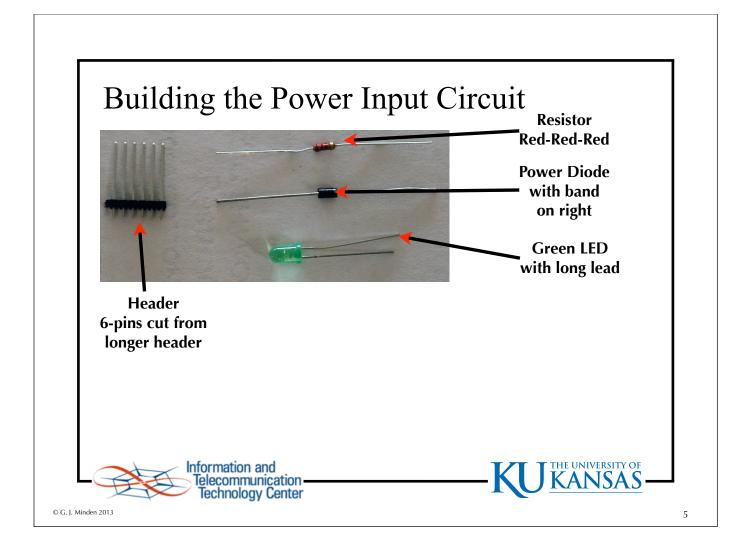
First, select a resistor, diode, LED, and header strip from your bag of parts.
